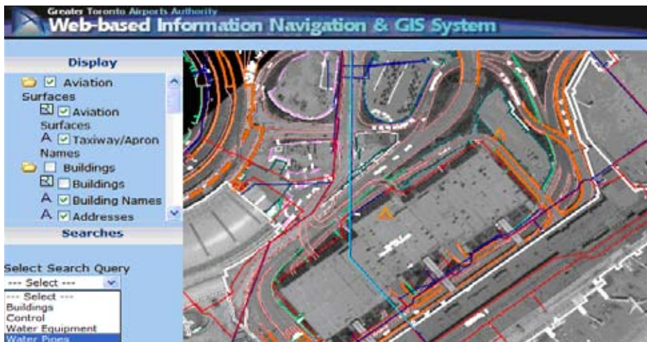
Fig. 5: The latest update of the TDC’s Map and data publishing portal dubbed “WINGS” utilizes Bentley Geo Web Publisher to provide on-line mapping services from CAD, Oracle Spatial and imagery data stores
