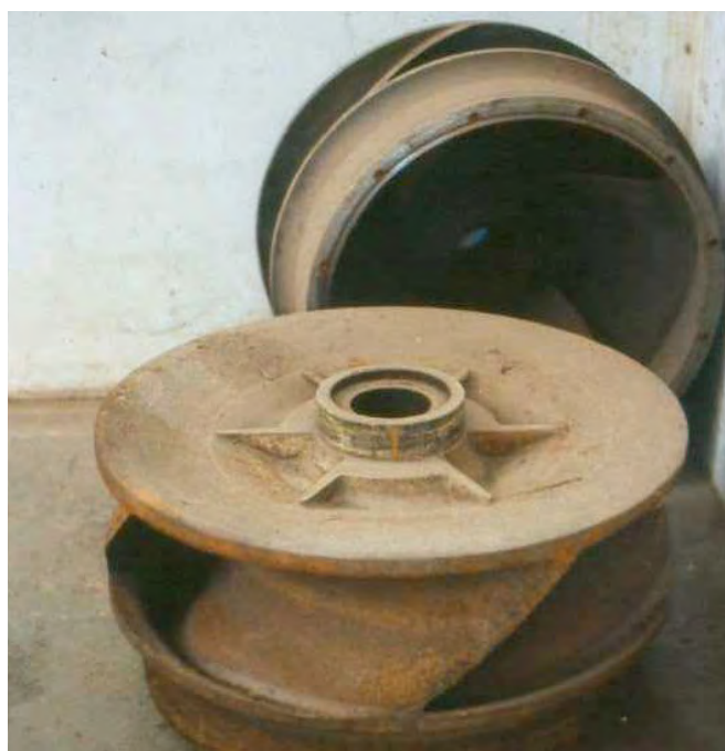
Sometimes, changing pump impellers can help to improve efficiency. Coating impellers also can improve efficiency, especially in large pumps.
