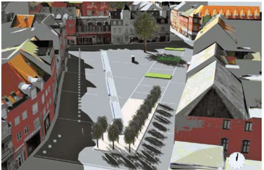
Unique to a 3D City GIS model, shadow analysis is used for visualising the impact new infrastructure has upon existing municipal structures. Courtesy BlomInfo A/S
