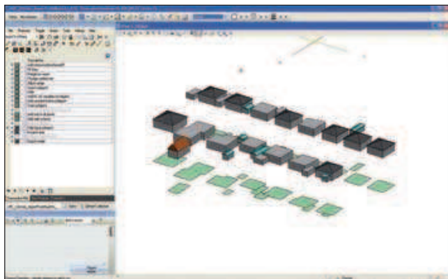
On-the-Fly 3D City and Urban Modeling of Odense Kommune, Denmark, BE INSPIRED winner in the category Innovation In Government. Bentley's GenerativeComponents product offers a parametric modeling capability that leverages GIS data to swiftly create 3D City models. Image courtesy of Bentley.
