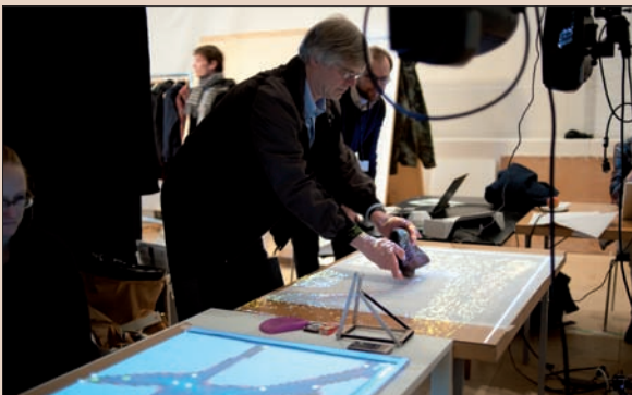
SmartGeometry co-founder Hugh Whitehead gets interactive on Ophelia's Beach. As physical objects are placed within the projected image their presence is detected by the Kinect sensor and fed into the virtual environment recalculating the wind flow around the new object in real-time.
