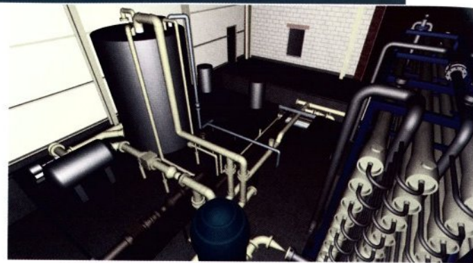
Figure 1A and 1B: Camp Dresser & McKee's master 3D model enabled numerous iterations, multiple design reviews, cross checks from other disciplines, and interference detection.
