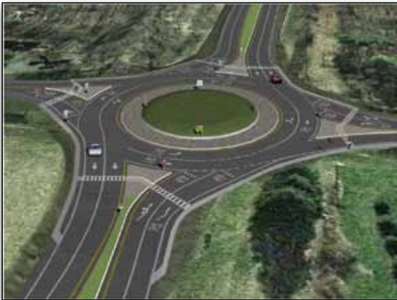
Designed with InRoads, this project by Creighton Manning Engineers features intelligent 3D modeling, machine controlled grading and stakeless construction and inspection.
