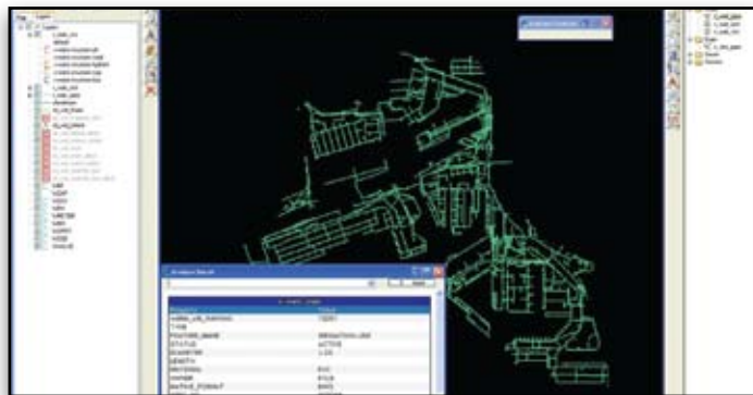
Bentley Map supports the mapping and analysis of infrastructure assets – in this case the port's water network.
