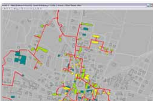
Bentley sisNET displays the district heating network and connected buildings.
