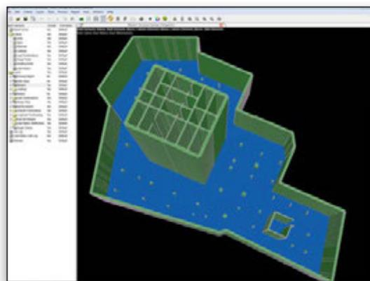
*Analysis and design of The Shard’s raft foundation in RAM Concept.*
