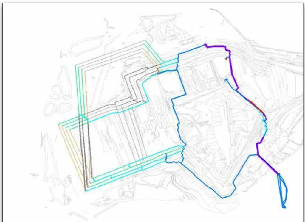
An example of modeling the mine fire service water system in WaterCAD.
