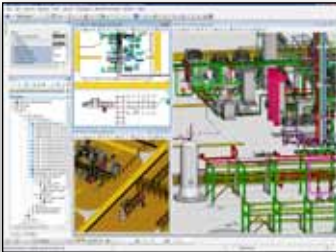
The Model Component browser provides a concise breakdown of the contents of the model repository
