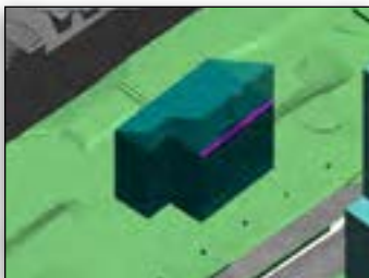
Extrude 2D building outlines into 3D features using push/pull solid modeling controls.
