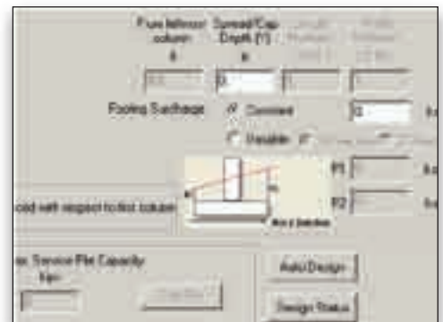
Variable Surcharge in Footing design: Users can define variable surcharge in both X & Z directions.
