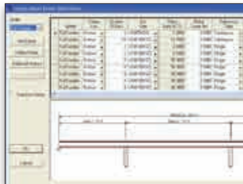
Rebar Dialog automates layout of mild reinforcement.
